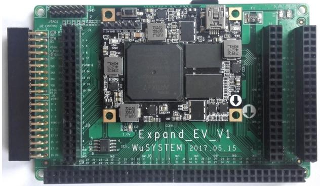
Figure 6: The FPGA evaluation board for  $\Phi$ PU and  $\Phi$ -Stack
